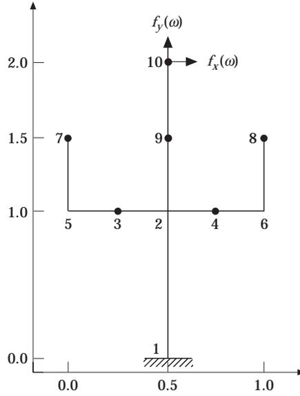
Figure 2. Geometry of the model FORK. Numbers indicate nodal points; ●, lumped mass; →, excitation.
